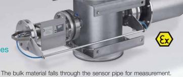
The bulk material falls through the sensor pipe for measurement. A representative partial flow is continuously fed to an optical measuring system and measured. The optics are protected by scratchresistant borosilicate glass and contamination is prevented by purge air.
